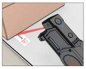
3. Use the Cubetape to scan the barcode on the ScanStik closest to the package. It may be easiest to scan down the package until the scanner reads the barcode on the ScanStik.
