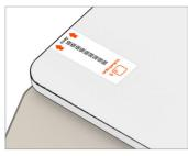
1. Peel the ScanStik and place it on an easily accessible reference edge - such as the side of the scale workbase.
