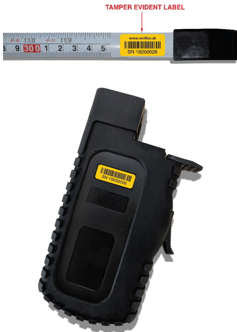
Figure 9 Alternative tape cassette sealing method (Alternative 7.5)
